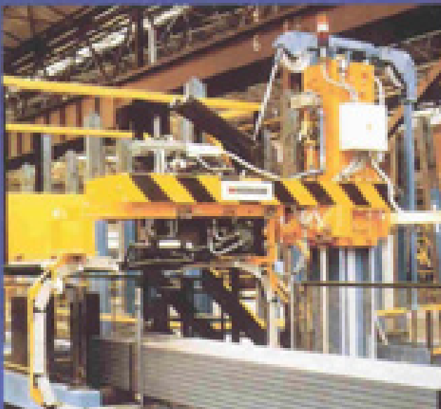
Fully automatic strapping of both hexagonal and square tube bundles.
