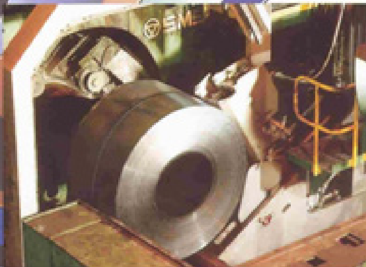
Sealless circumferential coil strapping.
