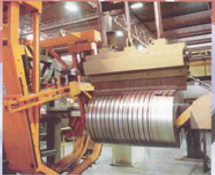
Automatic circumferential strapping of slit coils on a turnstile/capstan.
