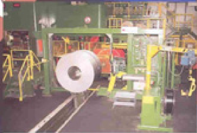
Strapping stainless steel coils on a cold roll reversing mill.
